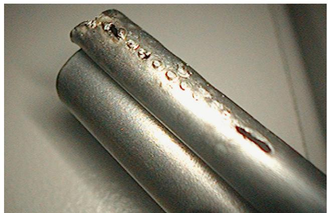
Fig. 3 – The KTP-laser is characterized by efficient PVP. However, applied to the metal sheet of the laser cystoscope or the tip of the optic the high energetic density could cause serious damage.
