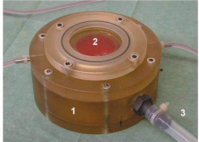
Fig. 1. Mechanical bioreactor with continuous perfusion of upper culture compartment (2) and air pressure (3) induced multi-axial stress performed on cell-matrix composite horizontally placed between the culture (2) and the pressure compartment (1).
